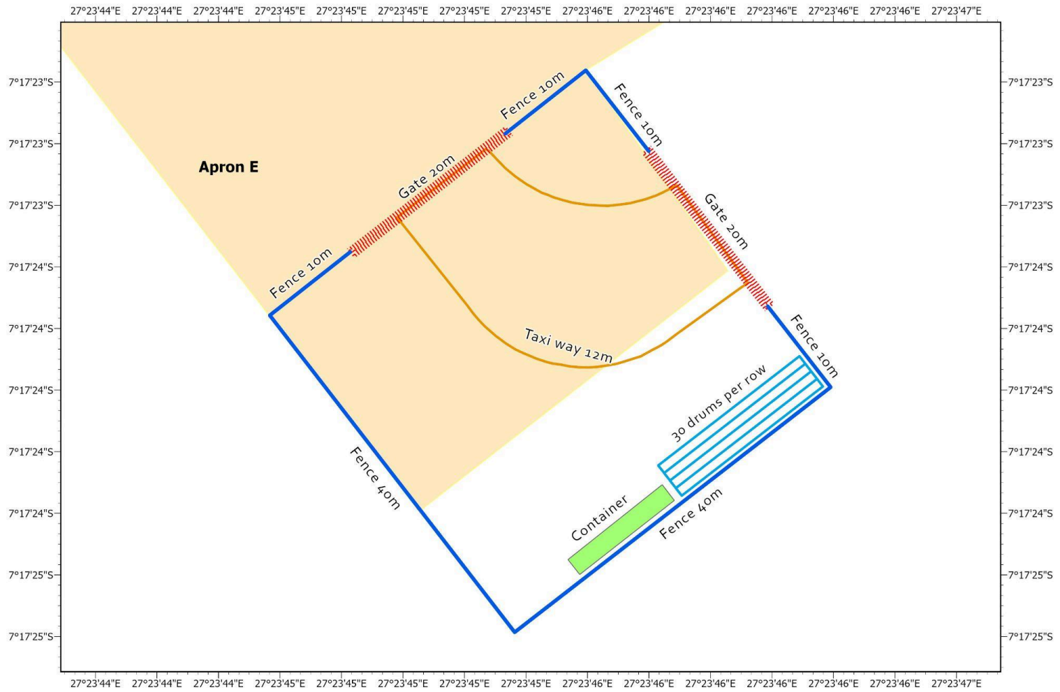
Figure 2: Above is an example schematic of the layout and recommended components of the airbase.
